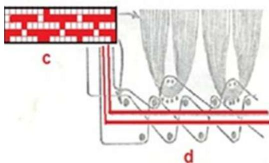
**Figure 5. Fabric structure and cross section of weft**
