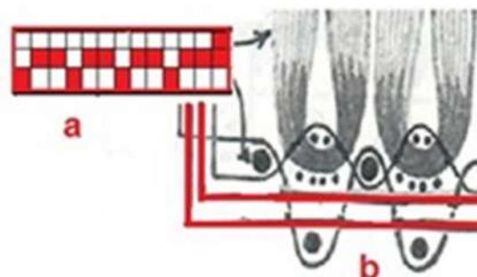
Figure 4. Fabric structure of Gauze and leno fabrics
